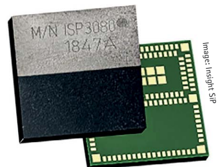
Figure 3: ISP3080 is a stand-alone solution for RTLS, access control, and indoor positioning applications.
