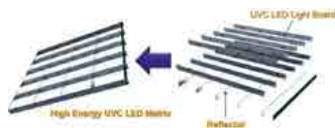
Figure 3: With three reflectors per UV-C LED, the matrix generates particularly high-energy UV-C radiation.
