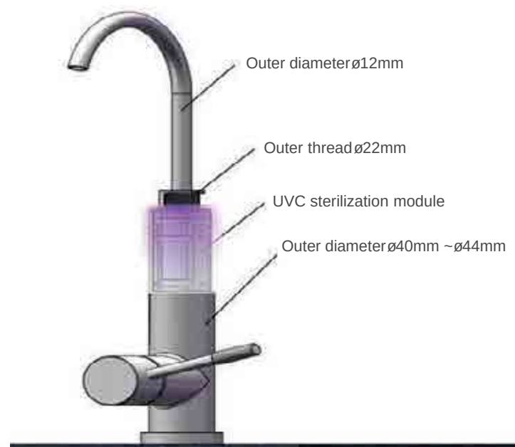
Figure 6: Germ-free water straight from the faucet: the Lextar faucet UV-C sterilization module, with a power consumption of 10 to 30 W, cleans at a flow rate of between 2 l/min. and 12 l/min.
