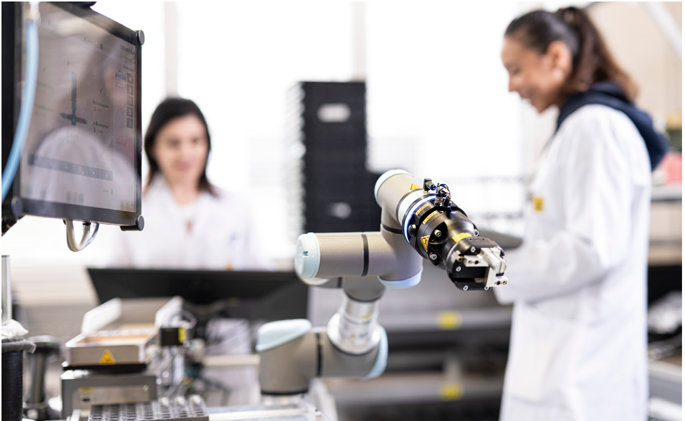
Cobots are specifically designed to work with an operator
